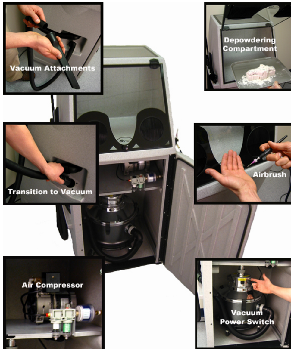
Figure 9: ZD5 Powder Recycling System
